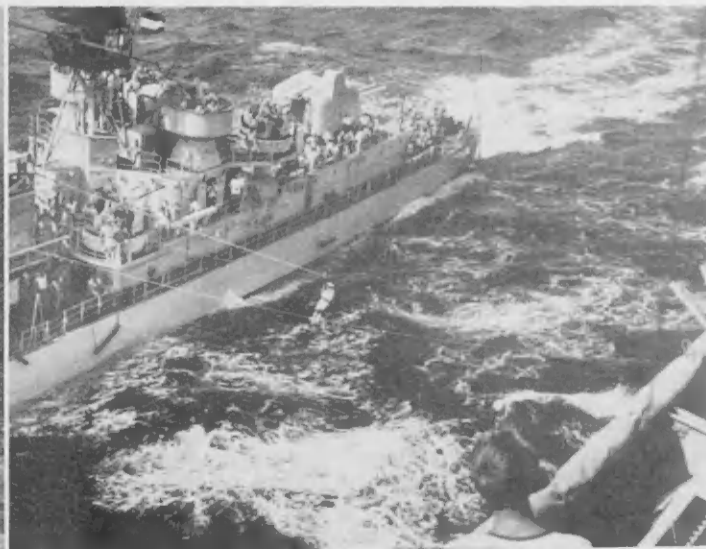
THE ESCORT HRMS Limburg accompanied the aircraft carrier in Caribbean waters. Alongside the carrier, a transfer of personnel was effected over lines connecting the two ships. E ESCORTE HRMS Limburg a acompaña e portaavion den awanan di Caribe. Canto di e portaavion un pasamento di personal a tuma lugar pa medio di linja.
